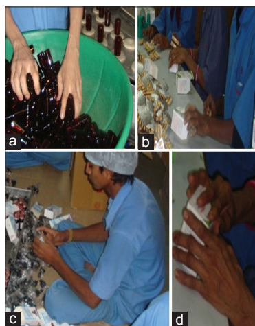
Figure 2: (a-d) Position of hand while picking up the water washed syrup bottles and arranging in dryer cum sterilizer. Picking up bottles and quality assessment of filled syrup bottles before packaging syrup and capsules packaging in plastic bags and box (both upper and lower)
